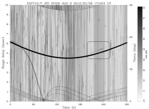
Figure 8. Range-time-intensity plot from the RAX-PFISR experiment conducted March 8, 2012. As in Figure 6, the strip of saturated signal is a side lobe from the direct radar pulses. Radar scatter from FAI is seen in the boxed region above the direct beam. The thin solid, dotted, and dashed lines show the aspect angles of scattering for the altitudes of 100, 200, and 300 km, respectively.
