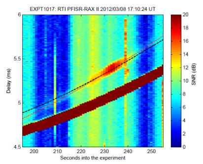
Figure 9. Zoomed-in portion of Figure 8 between 190 and 260 seconds. The black line is the expected range delay corresponding to FAI at an altitude of 100 km. The red line is a visual fit to the maximum intensity of the radar scatter.
