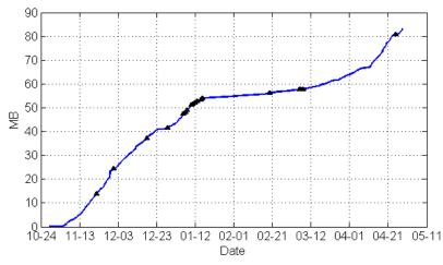
Figure 7. Cumulative sum of data received (MB) versus time. The markers in the plot indicate the dates that experiments were performed. By November 13, we were regularly downloading data. The lull around December 25 corresponds to a break for the holidays. The SD card failure on January 16 resulted in a much slower data collection rate due to the inability to schedule downloads.
