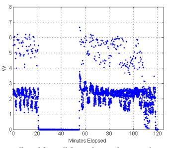
Figure 4. Sum of power collected from all four solar panels versus time, where time is minutes elapsed since 04 November 18:29:45 UTC. The portions with zero power collected are in eclipse. The data points with the higher power relative to the majority of data are when a beacon is transmitted. The power collection shown in this data is less than the full potential of the panels as minimal subsystems are turned on during this test.
