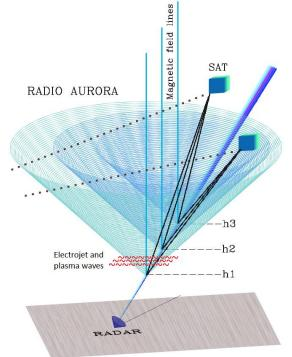
Figure 1. Drawing of the radar measurement geometry [4] [5]. The ground-based incoherent scatter radar station transmits pulses into the ionosphere, which scatter from the magnetic field-aligned plasma irregularities. The scattered signals are measured by the satellite-based radar receiver passing overhead. In the figure, the cones represent scattering from irregularities at three different altitudes. The cubes represent two passes of RAX-2.
