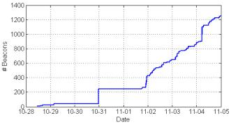
Figure 3. Cumulative number of beacons received over the first week of the mission. The steps in the data, such as at 10-31 and 11-2, are due to batch uploads to the database. Nominally, amateur radio operators use the publically available RAX ground-station client, and the beacons are automatically uploaded to the RAX database. Early in the mission, as the system was being deployed, there were some batch uploads rather than real-time uploads.
