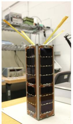
Figure 2. The RAX-2 flight unit.
