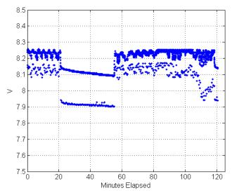
Figure 5. Battery voltage versus time for the same time period shown in Figure 4. As in Figure 4, the voltage points that are lower than the majority are when the radio is transmitting a beacon.
