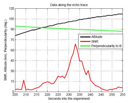
Figure 10. This plot shows FAI altitude, SNR, and aspect angle along the red line of Figure 9, which is a fit to the maximum intensity of the radar echo. Radar scatter was caused by FAI between the altitudes of 80 and 115 km. The angle shown in the plot is a measure of magnetic-field alignment. The maximum intensity of the scatter signals corresponds to an angle of 90°, where the Bragg wave vector is exactly perpendicular to the geomagnetic field lines.
