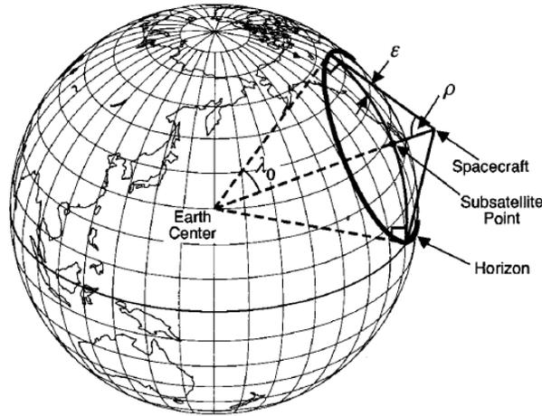
Figure 1. Geometric relationship between an orbiting satellite and a surface groundstation with respect to the center of the Earth. Figure used with permission.<sup>1</sup>
