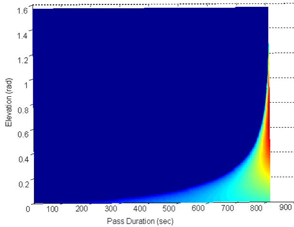
**Figure 6.** The total amount of data downloaded as a function of the elevation angle to begin communications and the pass duration. The more red the data point is, the more information that can be downloaded.
