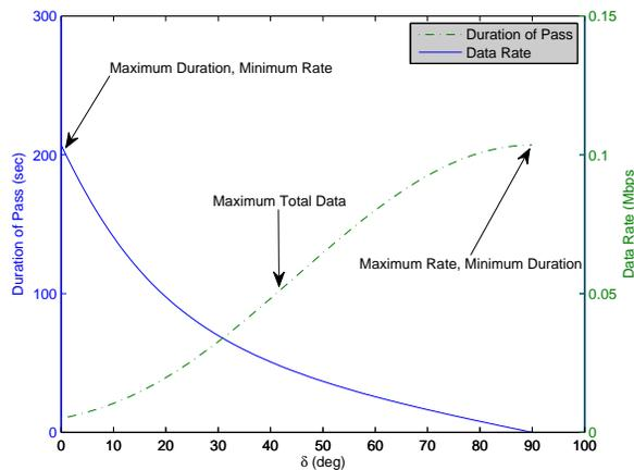
Figure 3. The data rate that can be maintained as a function of elevation and the corresponding pass duration for that data rate. For each elevation where communication begins ( $x$ -axis) the corresponding maximum data rate and duration of link can be found ( $y$ -axis). Orbit and satellite parameters can be found in Appendix A.
