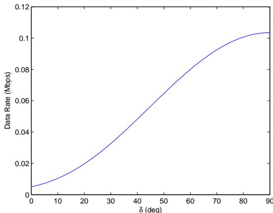
Figure 4. The data rate that can be maintained as a function of elevation,  $\delta_e$ . Here we assume the satellite passes directly over the groundstation. Orbit and satellite parameters can be found in Appendix A. It can be seen that significantly higher data rates can be achieved as the elevation increases, or equivalently, as the slant distance decreases.
