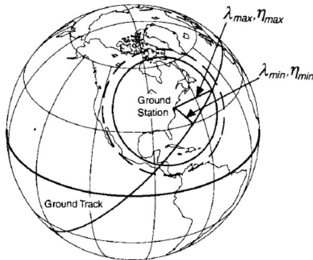
Figure 2. Geometric relationship between a spacecraft and the groundstation during a pass while on a circular orbit. Figure modified and used with permission.<sup>1</sup>
