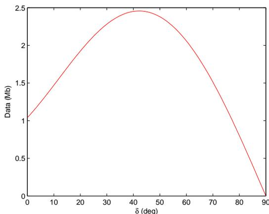
Figure 5. The total data downloaded as a function of elevation (data rate). For each elevation where communication begins ( $x$ -axis) the corresponding maximum data transferred can be found ( $y$ -axis). Note that a maximum exists at approximately 42 deg elevation. Orbit and satellite parameters can be found in Appendix A.
